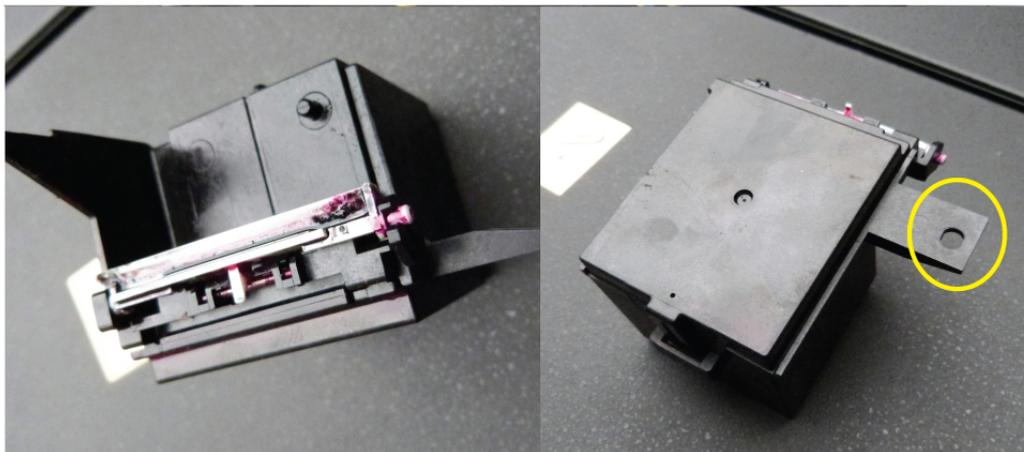
This is where you get a chance to look at the purge unit and pads but directly below the pads there is a black (Blade cleaner Unit box) If you examine this box closely you'll see two screws (Circled) they have to be removed to gain access to the purge unit waste pipe.
