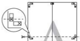
7. Lay the upper sheets on top of the lower sheets. The X marks should be matched as in the illustration below, and join the upper sheets and lower sheets together with cellophane tape temporarily.
