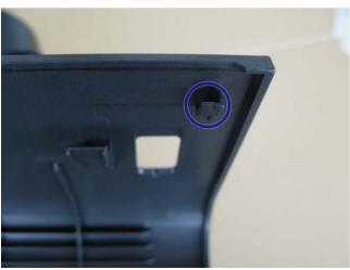
1) Remove the side covers (L and R) (no screws). < Release the claws on the top, then slide the cover down. >
