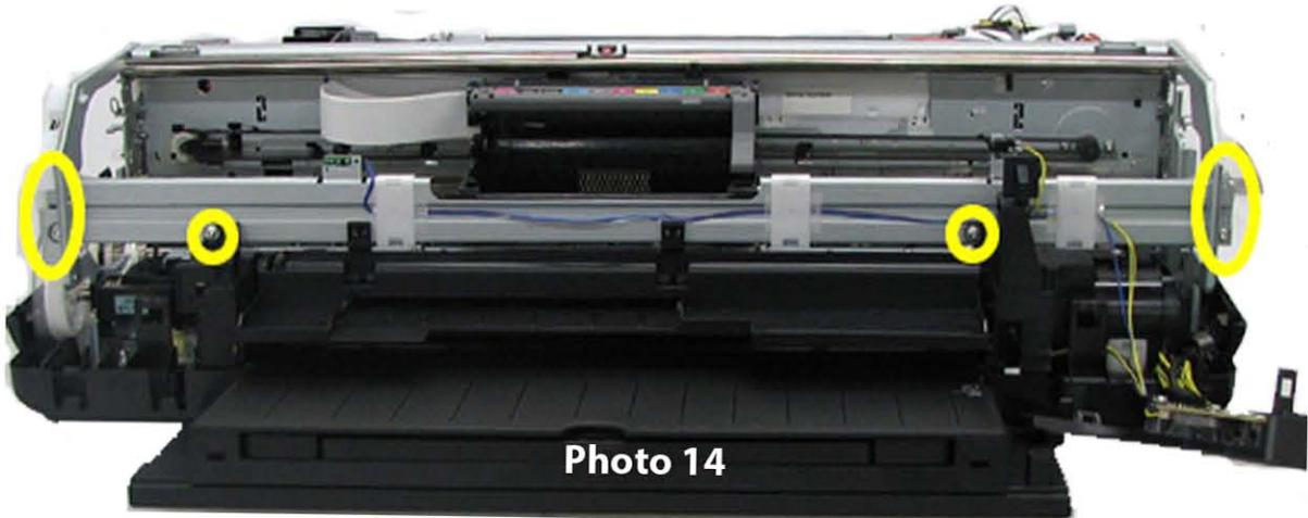
11. There are 2 screws on both ends of the stay (Bar), photo 15, 1 screw is hidden by white plastic Photos 16.
