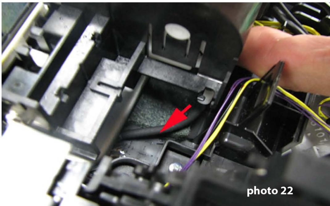
16. Photo 23. This is where the waste ink pipe is connect to the Purge Unit (Fig 1)
