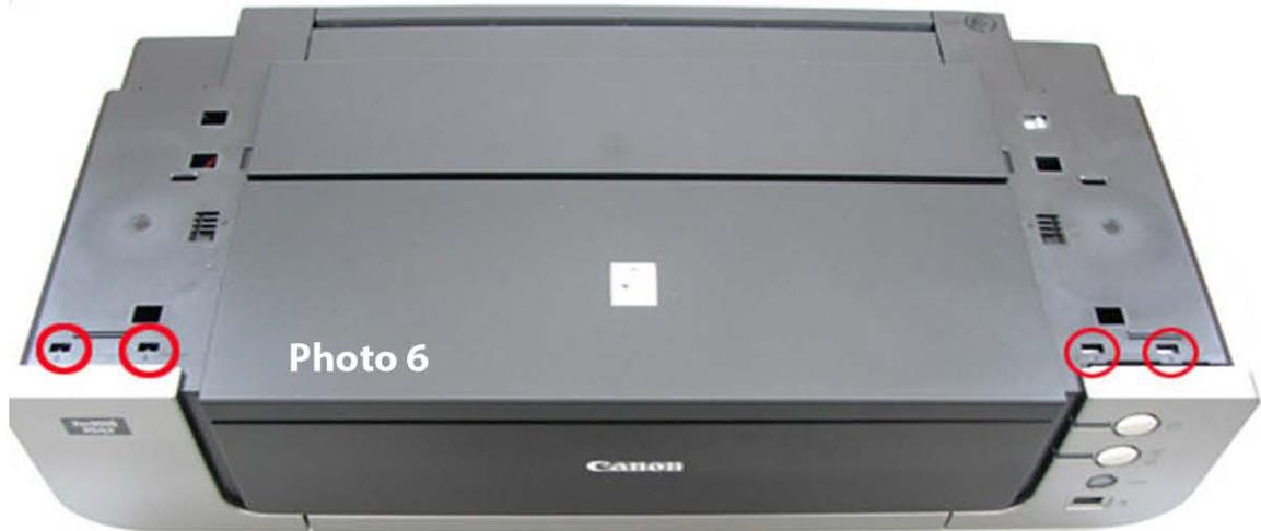
5. Use a screw driver to release the Claws on each Panel, (Photo 7 & 8 )
