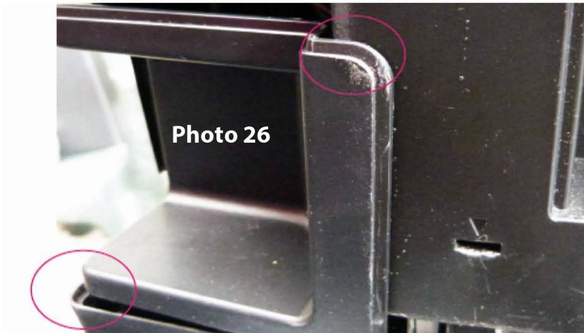
25. Then it's a matter of placing the top cover back over the printer once again and gently lowering into place but don't allow any claws to engage (Photos 10 to 13) before insuring the above corner piece is settle properly in photo 26 again.
