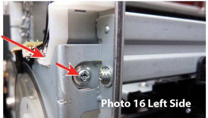
12. There are two remaining screws on the Stay (Bar).
