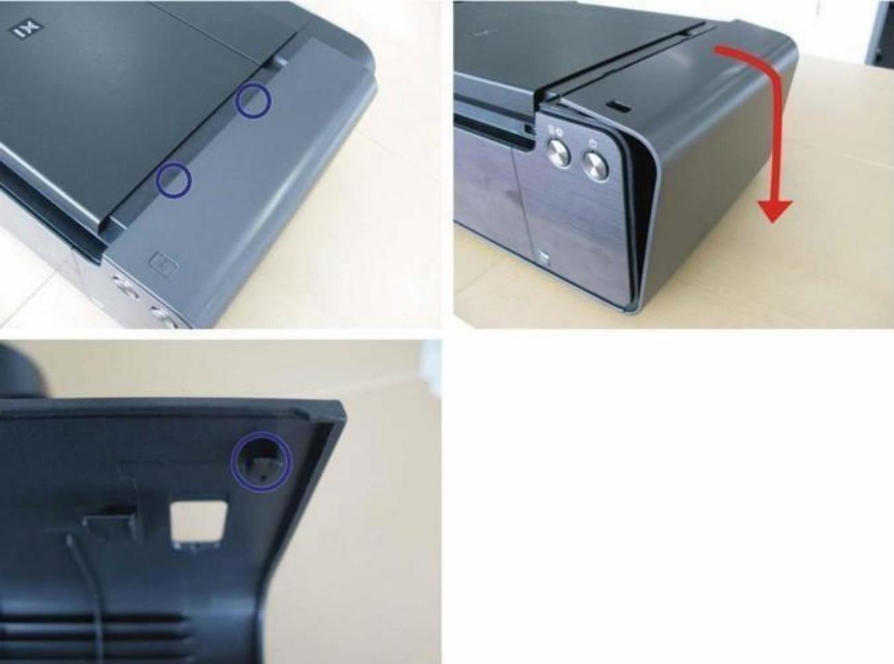
Be sure to protect the printer from static electricity in repair servicing, especially for the logic board, relay board, and PE sensor board. (1) External housing removal
