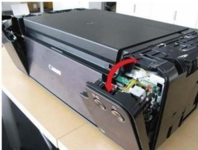
2) Remove the main case (no screws). < Release the claws of the tank door unit-SR (1 claw each), and open the tank door unit. >
