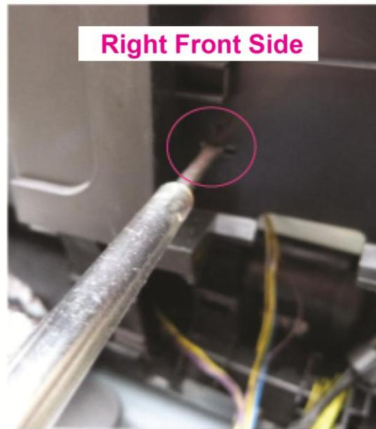
**These are the Pictures 7 & 8 Showing the Location of the Clips that are Holding on the Front of the Main Case Unit.**
