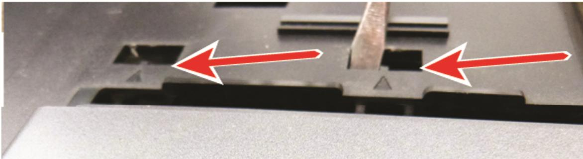
**Use the screw driver to release the Two front panel clips,
